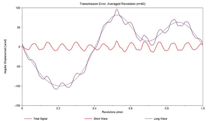
The transmission error curves show the deviation between the actual position of the driven wheel and the position it would occupy if the gearset were perfectly conjugate.
