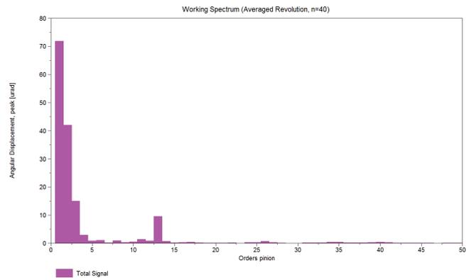
The spectrum of the total transmission error includes the tooth-meshing order, its harmonics and side bands.
